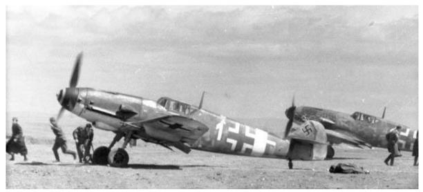
During their glory days flying against the Red Air Force on the Eastern Front, pilots of Luftwaffe JG 52 prepare for takeoff as ground crewmen remove chocks and head for cover. Note the 20mm cannon protruding from the nose of the Me-109.
