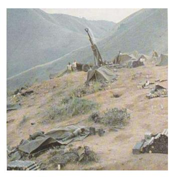
**HOWITZER:** an artillery cannon capable of both High-angle and Low-Angle fire. The 105mm howitzer was the most commonly deployed type in Vietnam, weighed about 5,000 lbs, and could fire a shell 11,500 meters (7 miles) at a rate of 3 rounds per minute. The 155mm howitzer was either a 2-wheeled, towed
