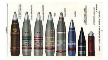
**SHELL-HE:** Shell carrying High Explosive. Explodes on the target causing damage by blast effect and by high velocity fragments (shrapnel). Typically the explosive was cyclonite (RDX), comprising about one half the weight of the shell.
