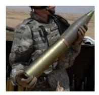
**SHELL:** The projectile, which carries a 'payload' to the target; fitted with a fuse on its nose to trigger its explosion. Payloads included high explosive, white phosphorus, illumination flares; smoke mixture, 'butterfly' bomblets, or anti-personnel fleshettes.
